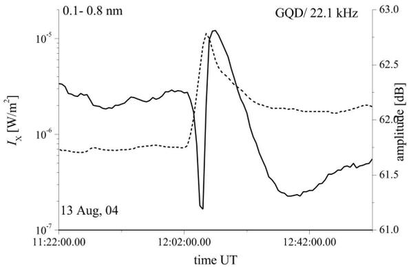
**Fig. 7.** Solar flare event (dashed line) with peak X-ray irradiance at 12:09 UT on 13 August, 2004 and corresponding disturbance of VLF signal amplitude (solid line). The characteristic events took place at time: 12:08 UT (first minimum), 12:12 UT (amplitude peak), and 12:35 UT (second minimum).
