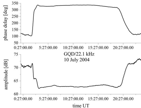
**Fig. 2.** Diurnal variation of the GQD signals amplitude and phase, during day without significant flares, 10 July, 2004. Universal Time is used. The amplitude is measured in dB over  $1 \mu\text{V/m}$ .
