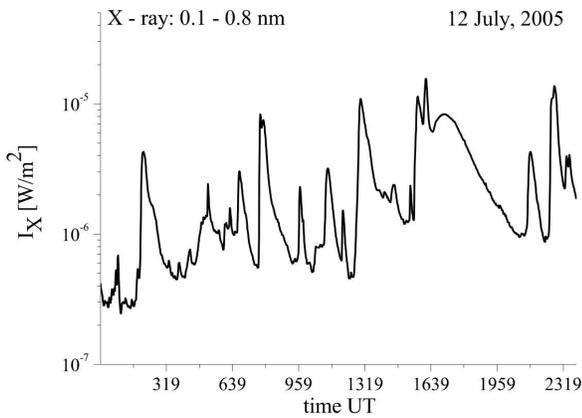
**Fig. 3.** Diurnal variation of the X-ray irradiance, on a very disturbed day, 12 July, 2005. Up to 15 significant flares, with  $I_X$  peaks exceeding  $10^{-6}$  W/m<sup>2</sup>, can be seen.
