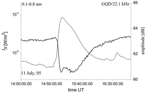
**Fig. 6.** Solar flare event (dashed line) with peak X-ray irradiance at 15:07 UT on 11 July, 2005 and corresponding disturbance of VLF signal amplitude (solid line). The characteristic events took place at time: 15:06 UT (first minimum), 15:10 UT (small amplitude peak), and 15:26 UT (second minimum).
