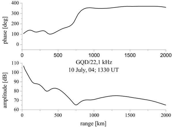
**Fig. 1.** The variation of the GQD/22.1 kHz signal amplitude and phase delay along the range of 2000 km on the great circle path, from Anthorn ( $54^\circ 53' N$ ,  $3^\circ 17' W$ ) to Belgrade ( $44^\circ 51' N$ ,  $20^\circ 23' E$ ) on the day without solar X-ray flares. Note the minimum mode of the amplitude at reflection point 750 km away from transmitter.
